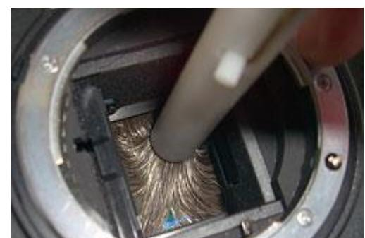
A brush used to sweep off and/or extract the dust. With some models the brush is energised to attract dust by blowing air through it creating a static charge, others are earthed to discharge the static that can cause dust to "stick" to the sensor.
